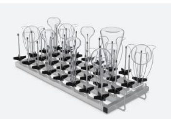
PLYT-32 32 positions cleaning bottle size:50-250ml PLYT-32 cleaning Erlenmeyer flasks, volumetric flasks, and flasks.With cross bottle holder and three-petal flower basket bottle holder.
